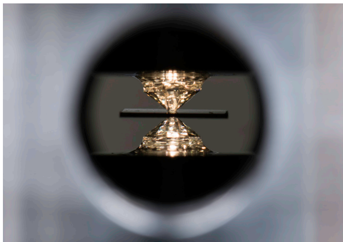
Crushed between two diamonds, a compound of hydrogen, sulfur, and carbon superconducts at room temperature. Photo courtesy of J. Adam Fenster/University of Rochester
