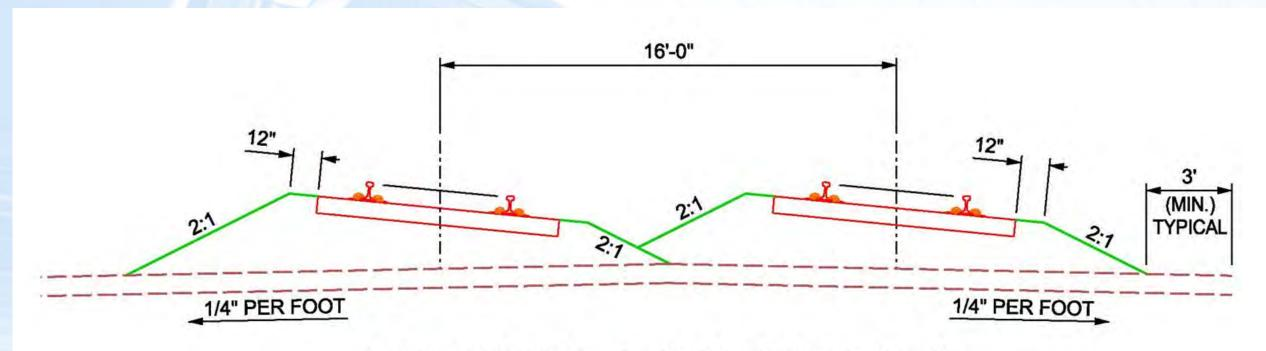
2 MAIN TRACKS - 5 1/2" SUPERELEVATION 16'-0" TRACK CENTERS
