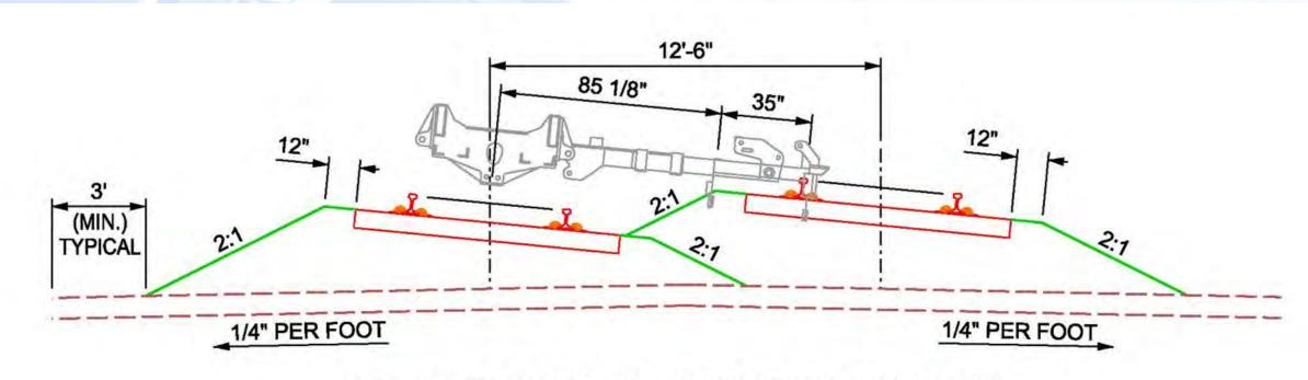
2 MAIN TRACKS - 5 1/2" SUPERELEVATION 12'-6" TRACK CENTERS - (6" HIGHER)
