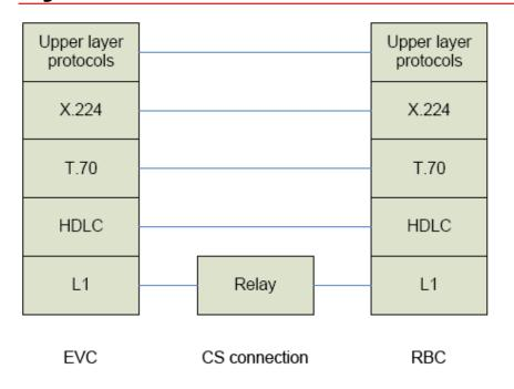
The protocol architecture according to the existing ERTMS specifications
