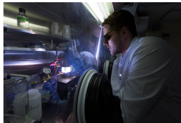
Preparation of U-Tc alloys by arc melting
