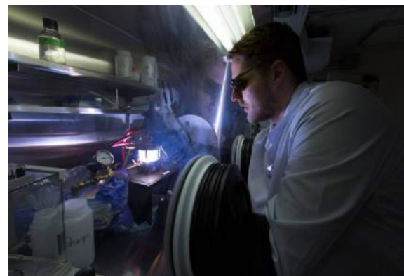
Preparation of U-Tc alloys by arc melting
