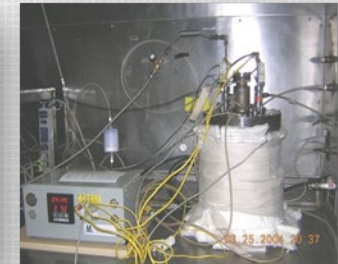
Yttria Stabilized Zirconia (YSZs) O 2 sensor for monitoring nuclear reactor coolant
