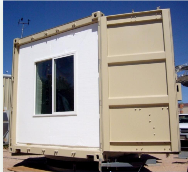
Figure 2. This photo shows the active side of the facility when a fenestration – the openings in the facility's walls – is being tested.
