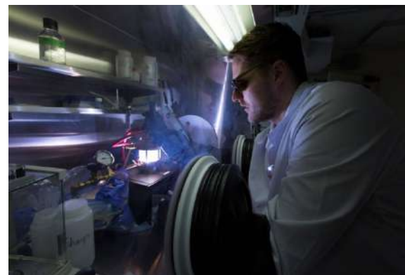
Preparation of U-Tc alloys by arc melting
