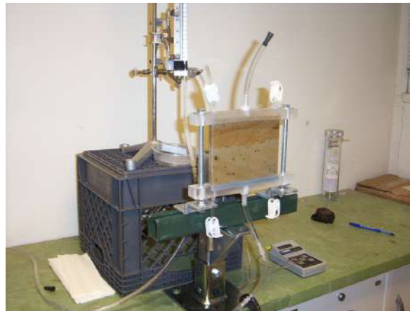
Hydraulic conductivity of a rock slab
