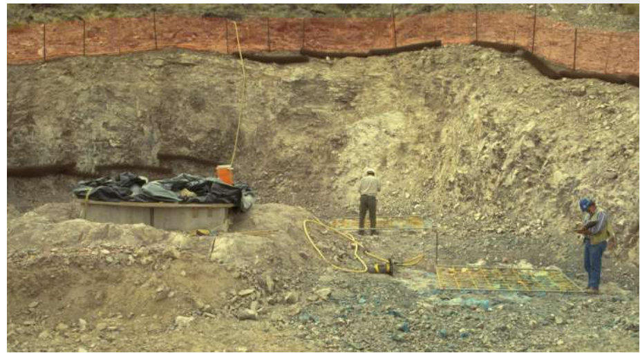
Field mapping of fracture networks blue dye (right foreground) is from an infiltration test
