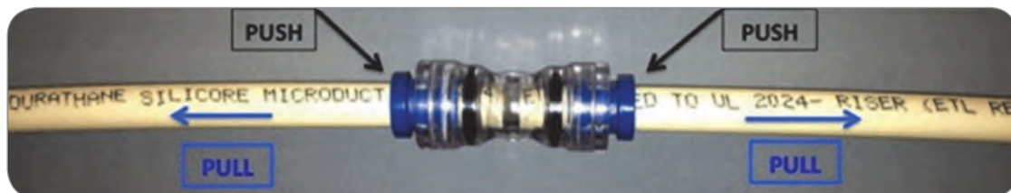
Remove coupler by pressing in on release rings (collets) and simultaneously pulling MicroDuct from the coupler.
