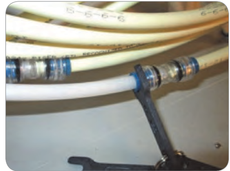
8.5 mm x 8 mm Transition Coupler (Part No. 1-907162)
