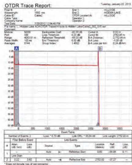
OTDR End-to-End Record Trace
