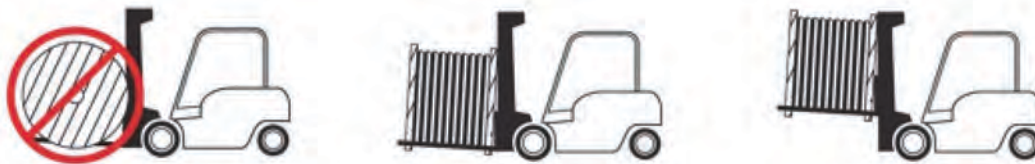
Lift reels by flanges to avoid damaging FuturePath.
