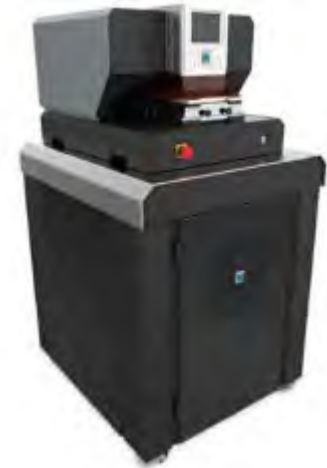
193 nm Excimer laser ablation system – Installed in 2021 to analyze mineral trace elements
