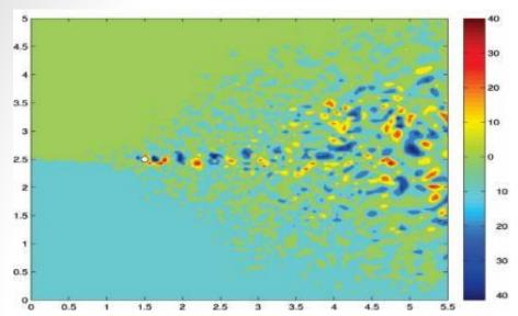
The figure (left side) presents the creation of the vortex street behind an immersed body in a fluid. It can be used to compute drag and lift in aerodynamics, such as drag and lift of aircrafts.
