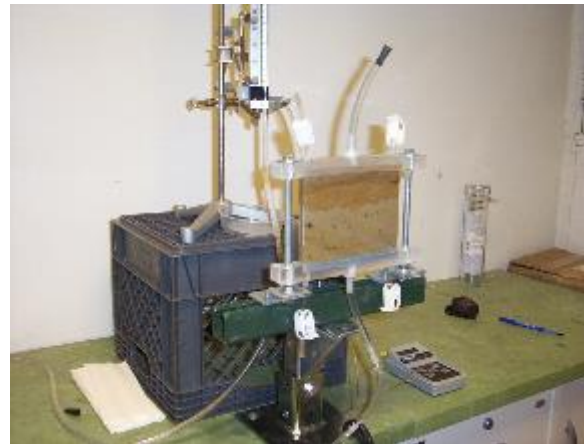
Hydraulic conductivity of a rock slab
