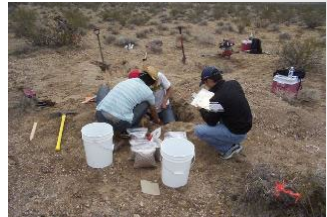
Sampling Chloride as a proxy for root-driven horizontal flow
