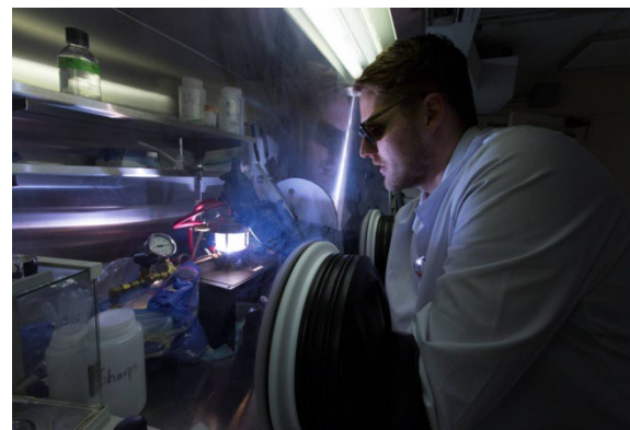
Preparation of U-Tc alloys by arc melting
