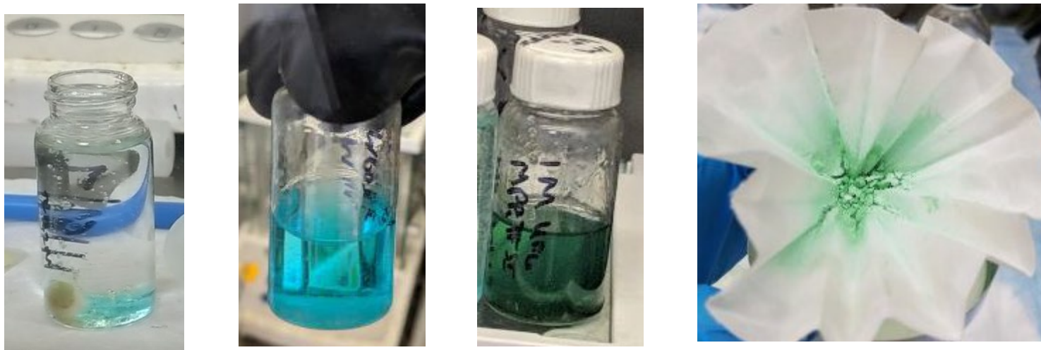
Dissolution of \text{UF}_6 into IL at 0 hours, 24 hours, 30 days, and the recovery of \text{UF}_6 salt.
