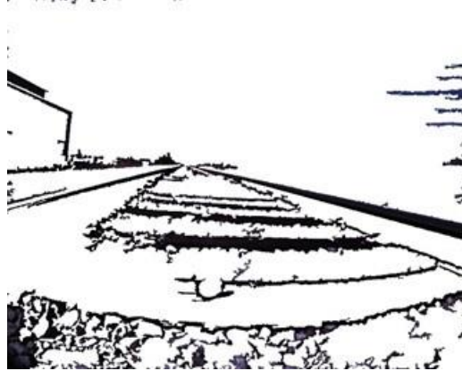
Figure 55 Canny edge detection-based method result.
