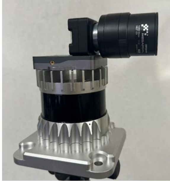
Figure 52 FLIR camera setup for data fusion
