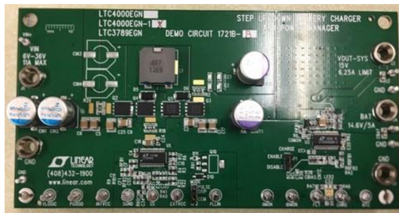
Figure 6-8. Commercial battery charging circuit demo board
