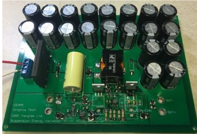
Figure 6-7. PCB of AC-DC and DC-DC (buck-boost) converter
