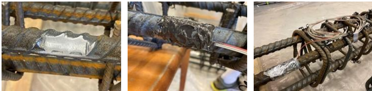
Figure 6.4 Strain gauge application
