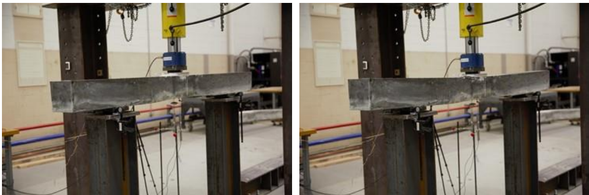
Figure 6.16 C468Ctie at start and end of loading
