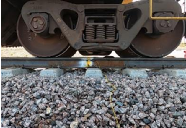
Welding defect 1: 0.8 in x 0.6 in. Location: 0.7 inches below the surface
