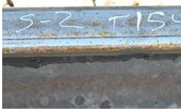
Figure 22 Rail crack in the web
