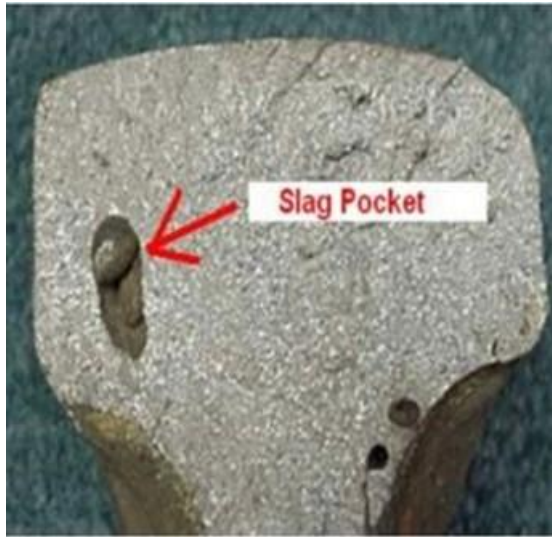
Defective weld with slag entrapment
