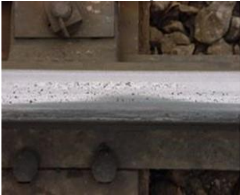
Flaking caused by centralized loading
