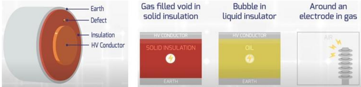
Figure 3 Causes of PD in switchgears and transformers
