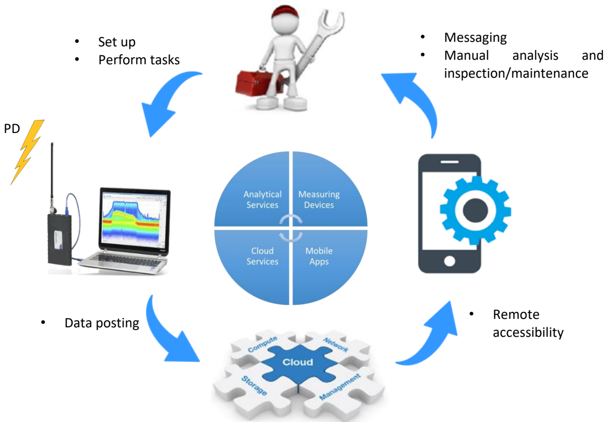
Figure 12 IoT-cloud-based remote real-time PD monitoring system diagram
