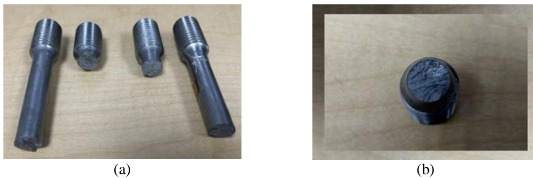
Figure 10.13 Failure shapes of the weld area samples
