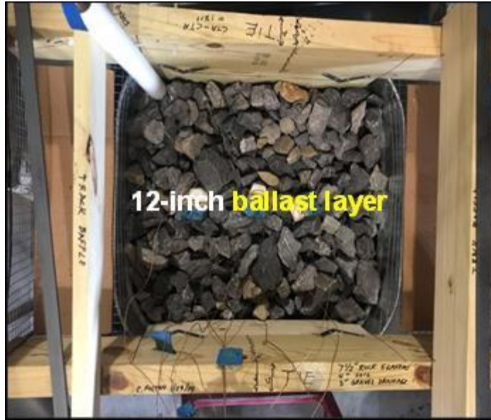
Figure 26. 12-inch deep ballast layer
