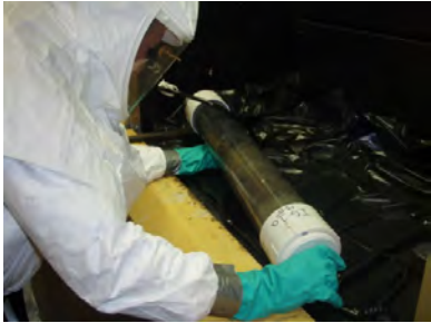
Contaminant Transport Studies – Column tests to determine flow and leachate from Superfund landfill sites
