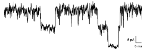
Patch clamp of single K + channels
