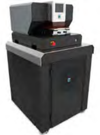
193 nm Excimer laser ablation system – Installed in 2021 to analyze mineral trace elements
