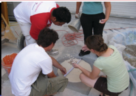
Figure 2: Slump Testing of Concrete Batch
