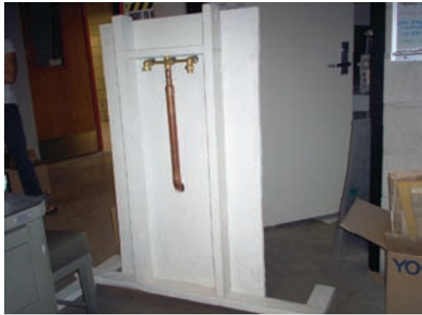
(upper) Elegant Bath Fountain front view, (lower) View from rear showing plumbing of one test case.
