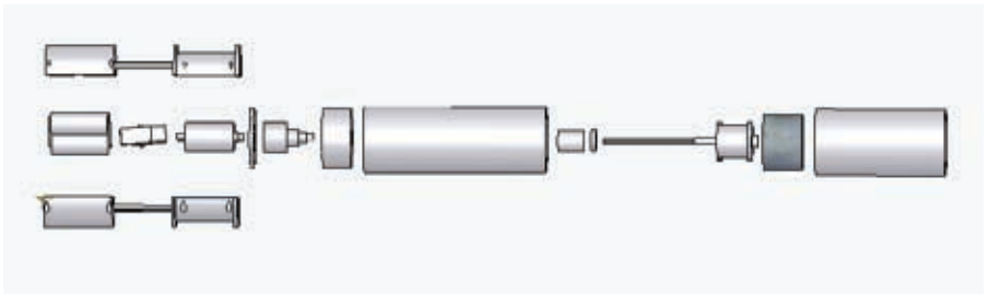
(upper) Photo of the functional prototype used in testing, (lower) Component view expansion of the new pepper grinder
