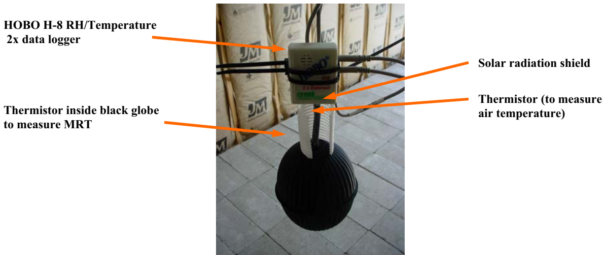
Fig. 7. Equipment Bundle Placed 43.3" (1.1 mts.) Above the Finished Floor
